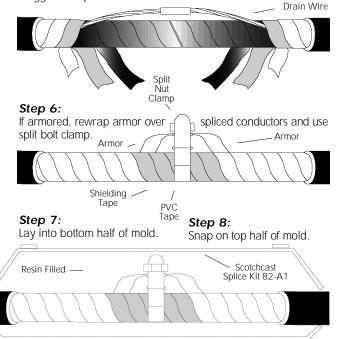
Step 9: Tape each end of mold to prevent resin from leaking out. Step 10: Insert funnels and pour resin to fill. Step 11: Remove funnels.
