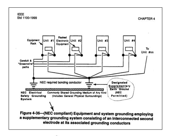
The bonding required by the NEC® can also be used for shielding purposes. By placing this wire above the major bundle of other wires and cables, a significant amount of lightning energy is absorbed and directed to the ground grids of the system. Here is a typical installation detail:
