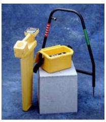
The 3M<sup>™</sup> 2273-U3P3 Advanced Cable, Metallic Pipe and Insulation/Sheath Fault Locator efficiently locates sheath faults and traces the path of underground cables, both copper and fiber optic (with metallic trace wire), and detectable tapes. Includes: Receiver, 3 Watt Transmitter, 3 inch inductive coupler, direct connect cable, and fault locating accessories. Paige Electric part number 270901.
